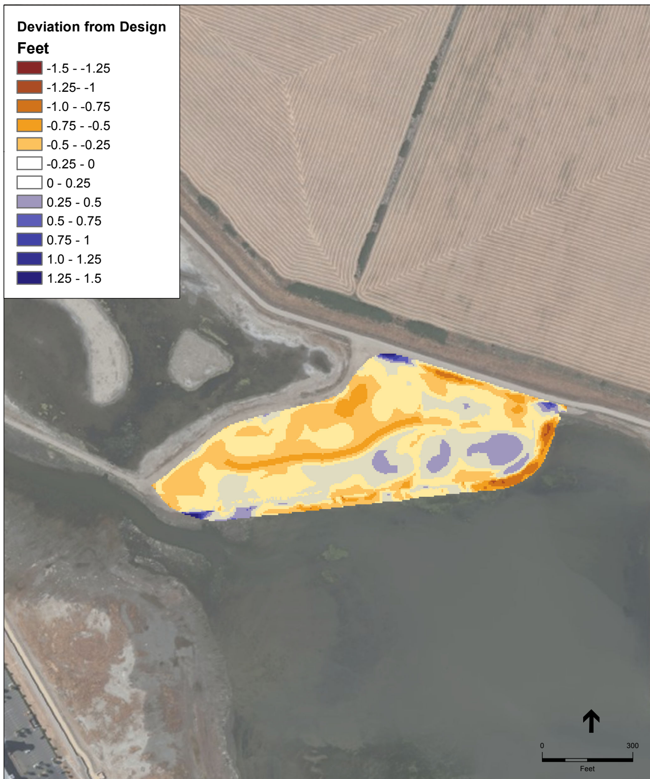
Hamilton - Post Construction . 1764.10 Figure 13 Tidal Panne February 2014 Post-Construction Point Survey vs Design Grade
